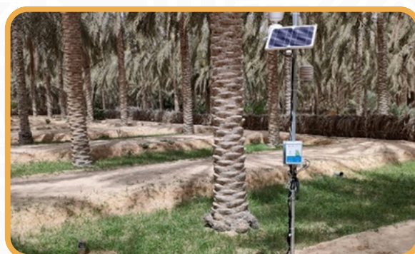
Picture: Irrigation control probe coupled with a weather station in Kebili (Tunisia)
